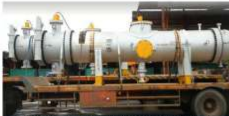
(MOC-CS+ SUPER DUPLEX STAINLESS STEEL CLADDED) INTER CONDENSOR FOR HGCL VISAKH REFINERY
